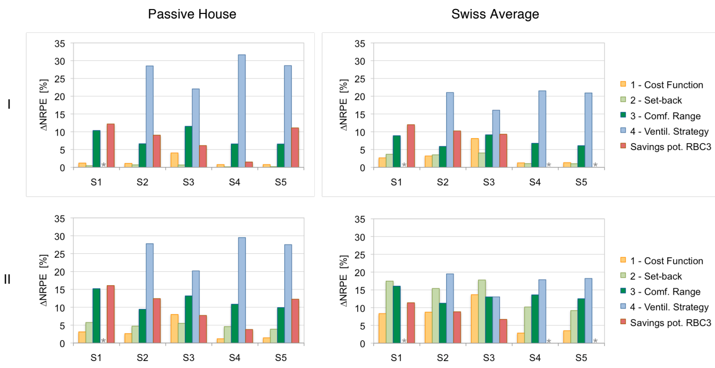
Figure 7.8: Comparison of average relative changes in annual total Non-Renewable Primary Energy (NRPE) usage due to variation in different factors (1–4) with average relative savings potentials for the rule-based control algorithm RBC-3 (cf. Table 7.11). I, II: Buildings Class; S1–S5: Building System variant; 1 – Effect of using alternative Cost Functions for control cost optimization and evaluation (cf. Table 7.5); 2 – Effect of allowance for night/weekend set-back (cf. Table 7.6); 3 – Effect of change in Thermal Comfort range width (cf. Table 7.7); 4 – Effect of different Ventilation Strategies (cf. Table 7.8). *: Value not available (Building System variant S1) or intentionally omitted (excessive thermal comfort violations, variants S4 and S5).
