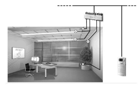
Integrated automation of light, blind, heating, cooling and ventilation
