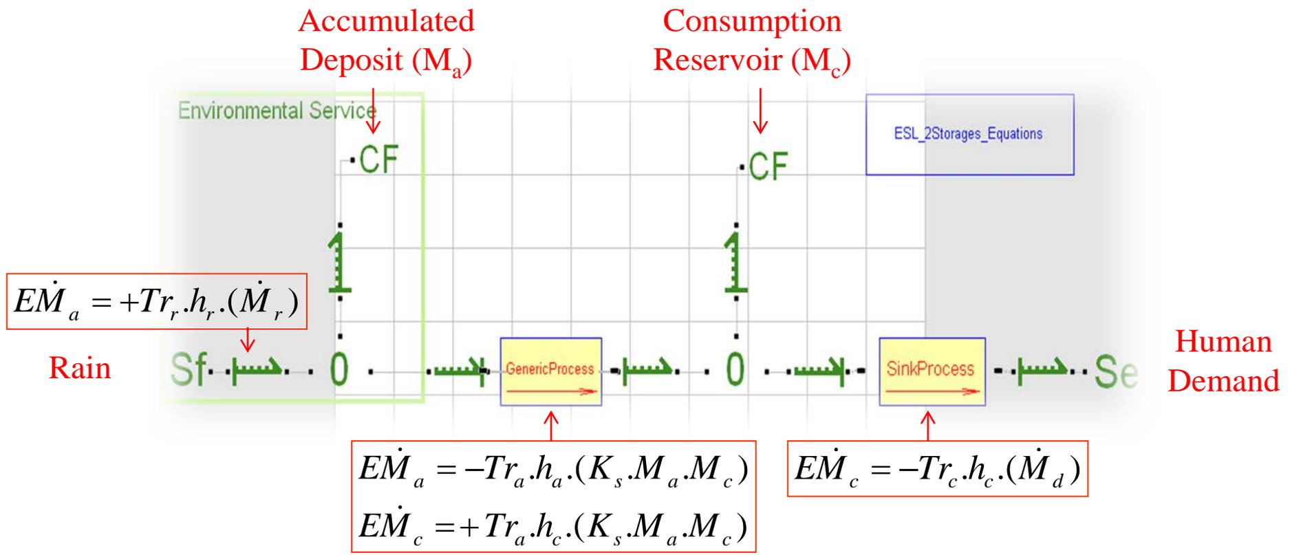
$$\begin{aligned} E\dot{M}_a &= Tr_r \cdot h_r \cdot (\dot{M}_r) - Tr_a \cdot h_a \cdot (K_s \cdot M_a \cdot M_c) \\ E\dot{M}_c &= Tr_a \cdot h_c \cdot (K_s \cdot M_a \cdot M_c) - Tr_c \cdot h_c \cdot (\dot{M}_d) \end{aligned}$$
