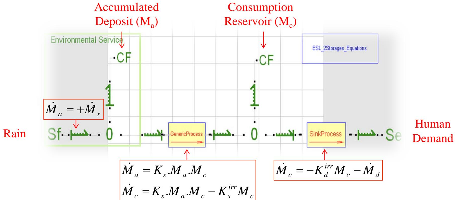
$$\begin{aligned} \dot{M}_a &= \dot{M}_r - K_s \cdot M_a \cdot M_c \\ \dot{M}_c &= K_s \cdot M_a \cdot M_c - K_s^{irr} M_c - \dot{M}_d \end{aligned}$$
