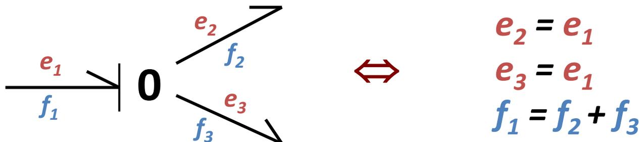
*Junctions of type **0** have only one flow equation, and therefore, they must have exactly one causality bar.*
