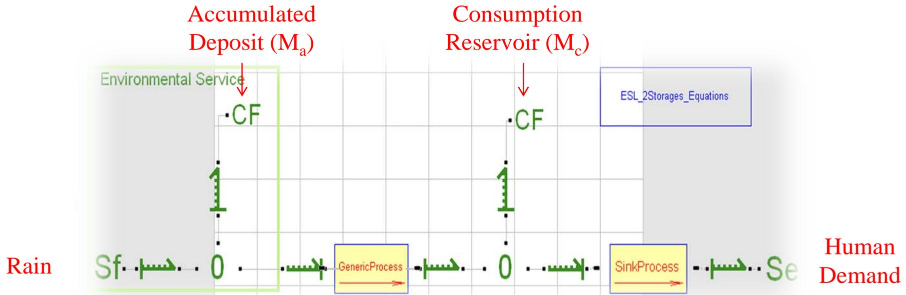
$$\begin{aligned} \dot{M}_a &= \dot{M}_r - K_s \cdot M_a \cdot M_c \\ \dot{M}_c &= K_s \cdot M_a \cdot M_c - K_s^{irr} M_c - \dot{M}_d \end{aligned}$$
