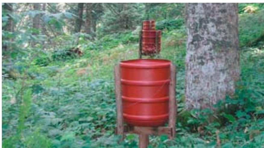
Litterfall traps installed at a fir Level II plot in central Greece.
